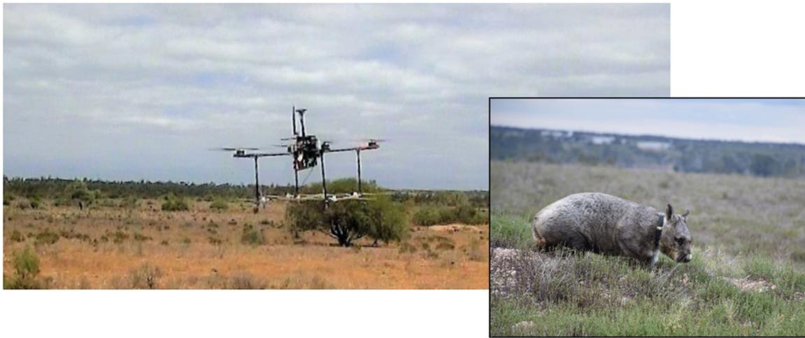
**FIGURE 1** A ConservationBot in flight, right after take-off to track and locate southern hairy-nosed wombats. Inset: Southern hairy-nosed wombat *Lasiorhinus latifrons* released into their habitat after being tagged with a very high frequency radio collar.
