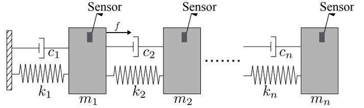
Fig. 1. An  $n$ -DoF structural system.
